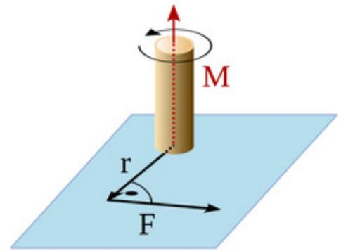
If a force  $F$  acts on an object with a fixed rotation axis, this object has the tendency to rotate. The greater the distance  $r$  of the force from the axis, the higher the torque. Torque generally is defined by the vector product. If the force is perpendicular to the rotation axis, and if  $r$  is the vertical (shortest) distance between the axis and the line of action of the force, the formula can be simplified to  $M = r \times F$ ; unit: newton metre.
