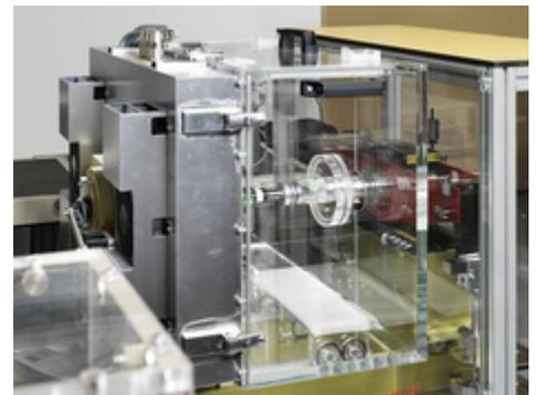
Customised Memmert climate chamber in the standard torque measuring instrument at the PTB
