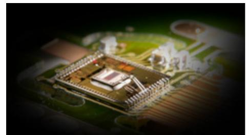
Fig. 3: Wire-bonded die-on-die module
