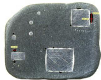
Fig. 1: Polish through the epoxy resin and the seven integrated circuits; after curing the epoxy resin without treatment in the vacuum drying oven 10 big voids are visible
