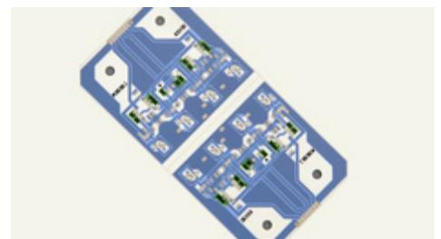
Fig. 4: Thick film substrate
