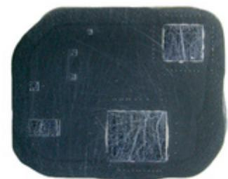
Fig. 2: Polish through the epoxy resin and the seven integrated circuits; curing of the epoxy resin after degassing in the vacuum drying oven results in a void-free structure; the cross-sections of the wire-bonds are well visible as small metallic dots in the epoxy resin
