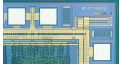
Fig. 5: Corner of a Microdul integrated circuit
