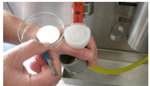
Filter membrane for the residual contamination analysis of components
