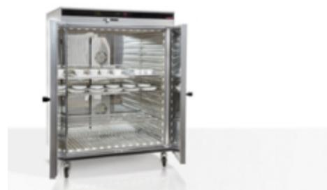
Memmert air-circulation heating oven UFP800DW for tests in accordance with DIN EN 50242/DIN EN 60436
