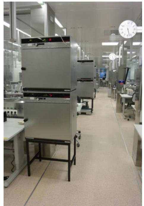
MED-EL cures adhesives and silicone in a Memmert drying oven.
