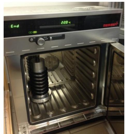
Adhesive bonds between the strain gauges and crank spider are dried in the Memmert drying oven
