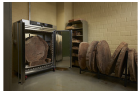
Memmert UF750plus drying oven for determining the density of wood
