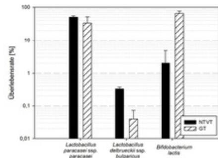
Maximum survival rates of diverse bulgaricus strains with a residual humidity of 6 to 7 %, depending on the drying process applied (low temperature vacuum drying (LTVD) and freeze drying (FD) ) [2]
