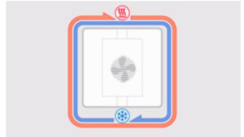
Air jackets around the interior of a cooled incubator prevent samples from drying out
