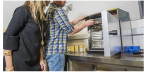
Test to determine the compression set as per ISO 1856 in the Memmert heating oven.
