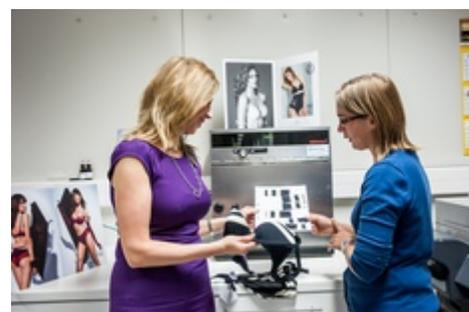
Memmert heating oven UNB200 for the testing of colour fastness of textiles
