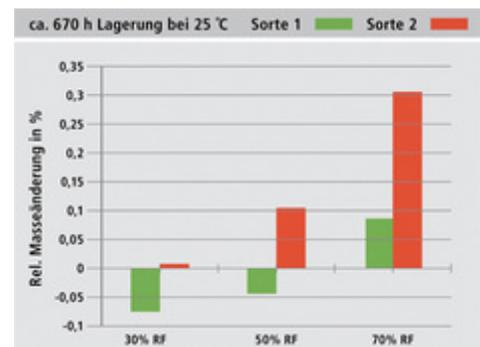
Figure 1: change in weight in carbide types 1 and 2 during long-term storage at different levels of humidity
