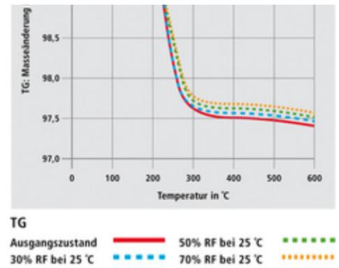
Figure 2: change in weight in carbide type 1 during the sintering process
