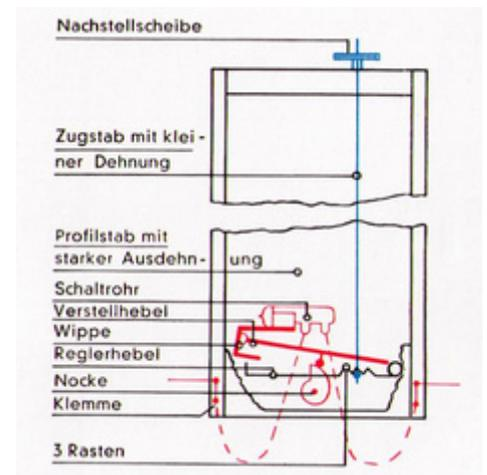
Fig. 4: Scheme of **Willi Memmert's** mechanical controller (dated back to the 60s)
