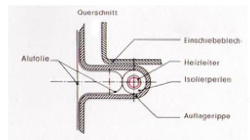
Fig. 5: Cross-section through a hollow in the inner chamber, with integrated heating element
